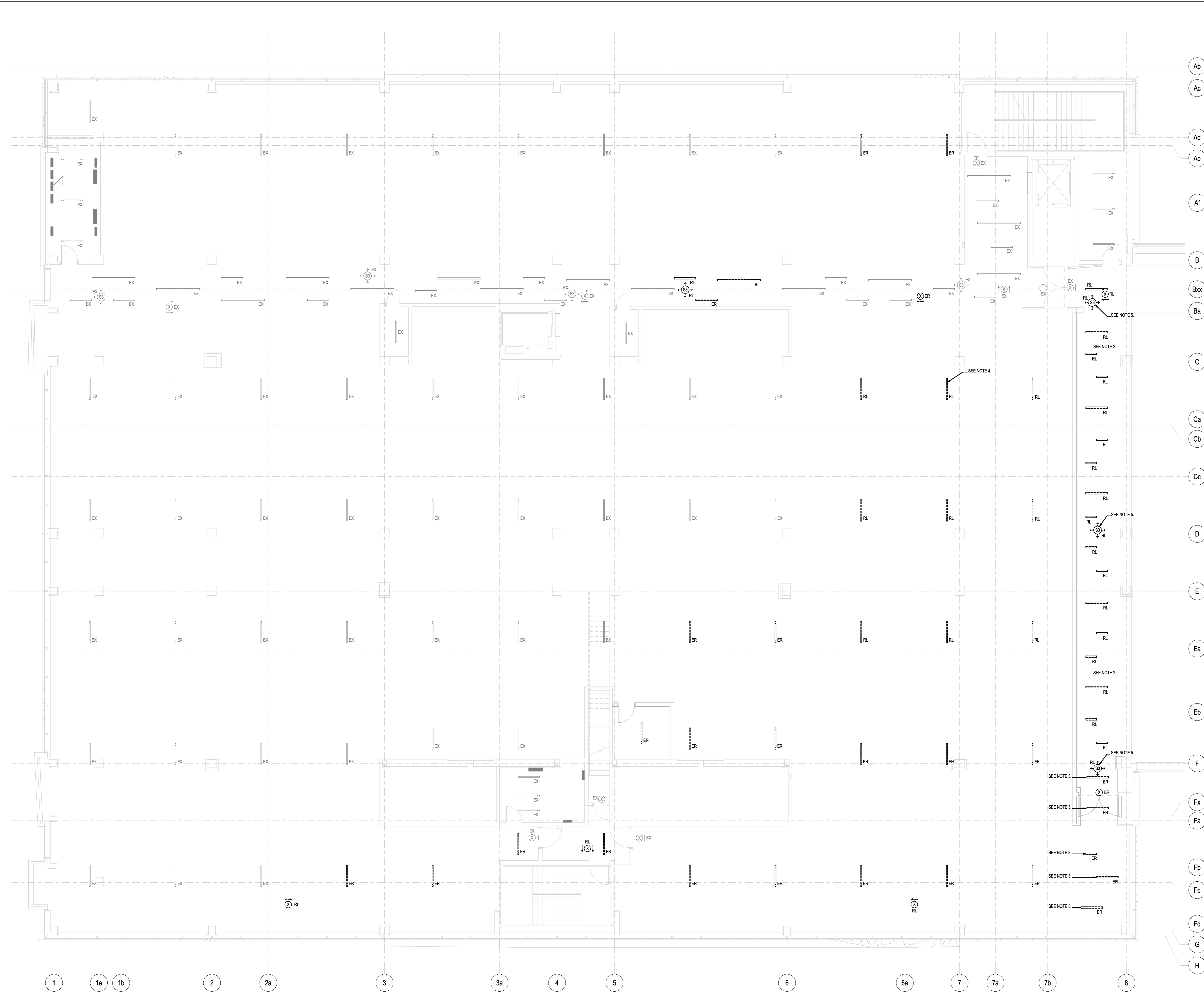
1 DEMOLITION LIGHTING FLOOR PLAN - LEVEL 5 PAV-A SHELLED SPACE E101 1:75
